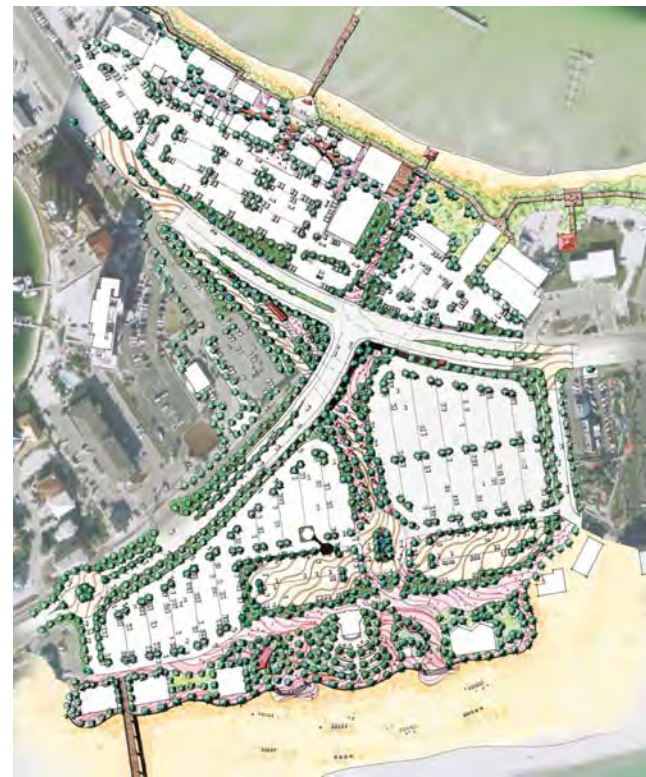
Concept B - Elevated Roadway with At-grade Pedestrian Concourse and Beach Access Road
